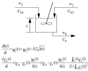
Where h (t) is the liquid level, Cb (t) is the product concentration at the output of the process,  $w_1$  (t) is the flow rate of the concentrated feed Cb<sub>1</sub>, and  $w_2$  (t) is the flow rate of the diluted feed Cb<sub>2</sub>.
